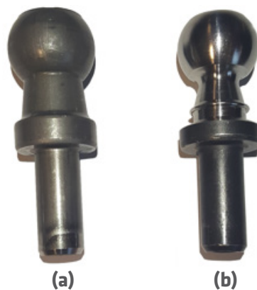
Fig.7 (a) Preform by cold forging, (b) final form by machining.
