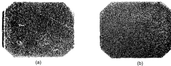
Figure 3. Surfaces of WC/Co samples after EDM-cutting with (a) one pass and (b) three passes.
