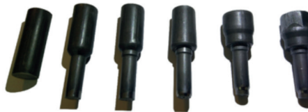
Figure 9. Stage designs and final product obtained from the production.
