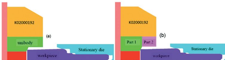
Figure 6. Schematic representation of the moving design of fourth stage; (a) Current design, (b) Split design. Part 1 and Part 2 are the split moving dies.
