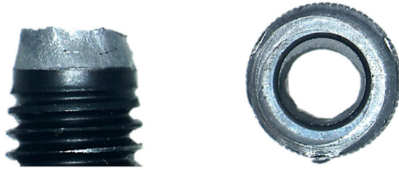
Figure 11. Fatigue failures observed from the head region.
