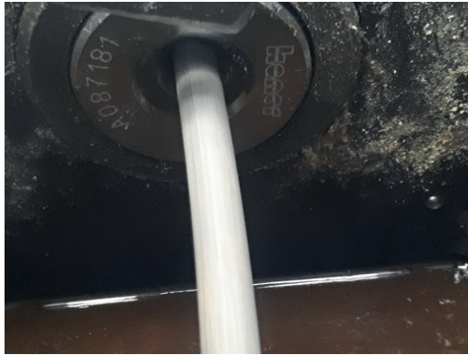
Figure 11. Wire surface condition after wire-drawing operation with redesigned die.
