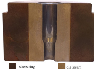
Figure 1. Typical cold forging die system consisting of insert and stress ring.
