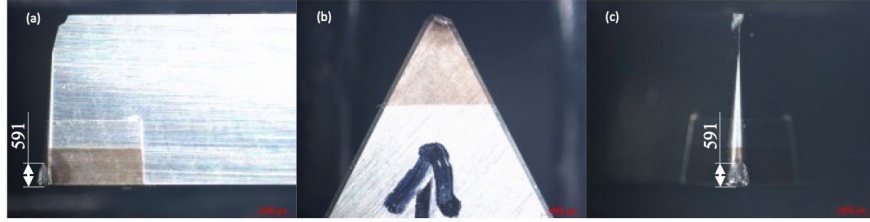
Figure 2. (a) Flank, (b) nose and (c) top view of an insert after cutting operation.
