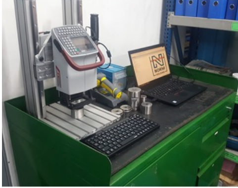
Fig. 3. Portable dot peen marking printer with a stand located in die warehouse.
