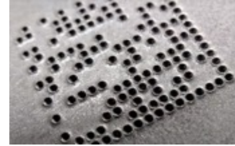
Fig. 4. QR code printed with a dot peen marking printer.
