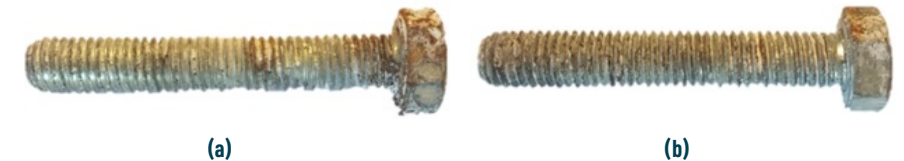
Fig. 4. Bolts after salt spray test; a) Zn_{Cr^{+3}} b) Zinc flake. The length of the bolts is 50 mm.
