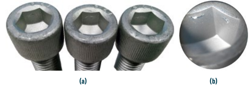
Fig. 2. a.) Burr formation in Allen bolts; b.) Close-up of burr formation in hex-socket of M20 DIN 912 Bolt.
