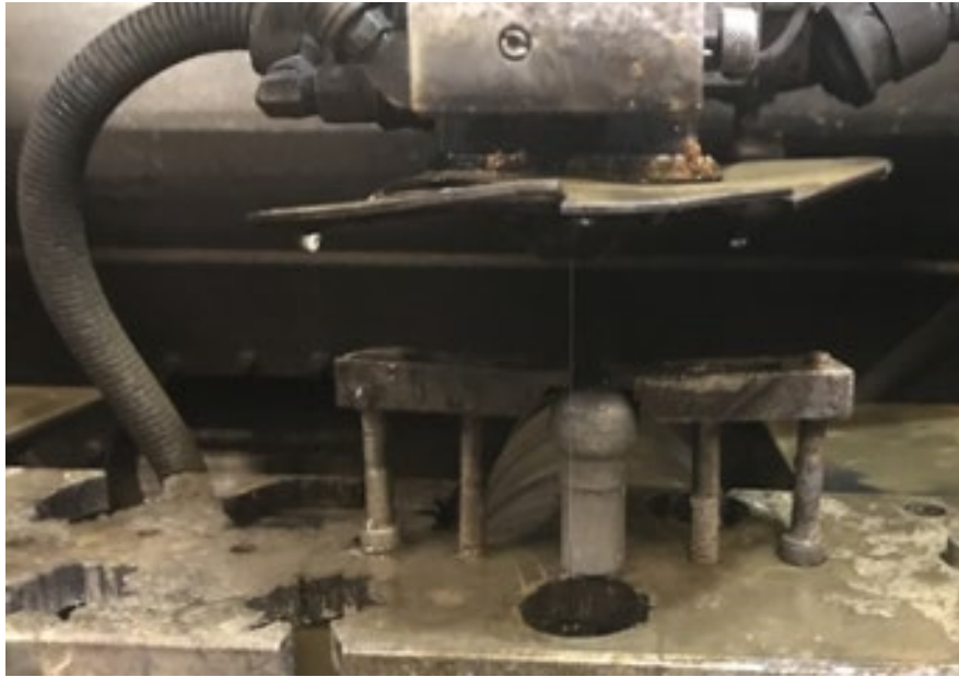
Fig. 4. Cutting configuration employed for the contour method.
